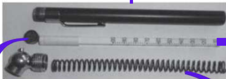
(c) Photograph of the components within a pencil-type pressure gauge
